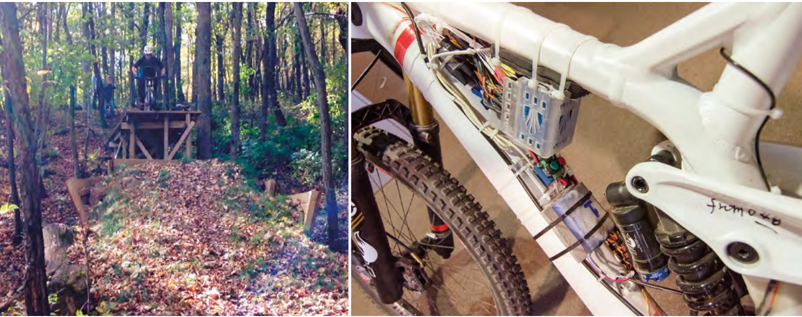
Figure 1. (Left) The Abaqus/True Load simulation used two extreme events to test drive the bike's load cases: Deer Hunter (shown above: a bike and rider poised to drop from a raised platform down to the ground) capable of fully compressing the rear suspension, and Mojo, a jump that did the same but also allowed the rider to rotate the bike. Figure 2. (Right) Strain gauges attached onto a bike frame.
