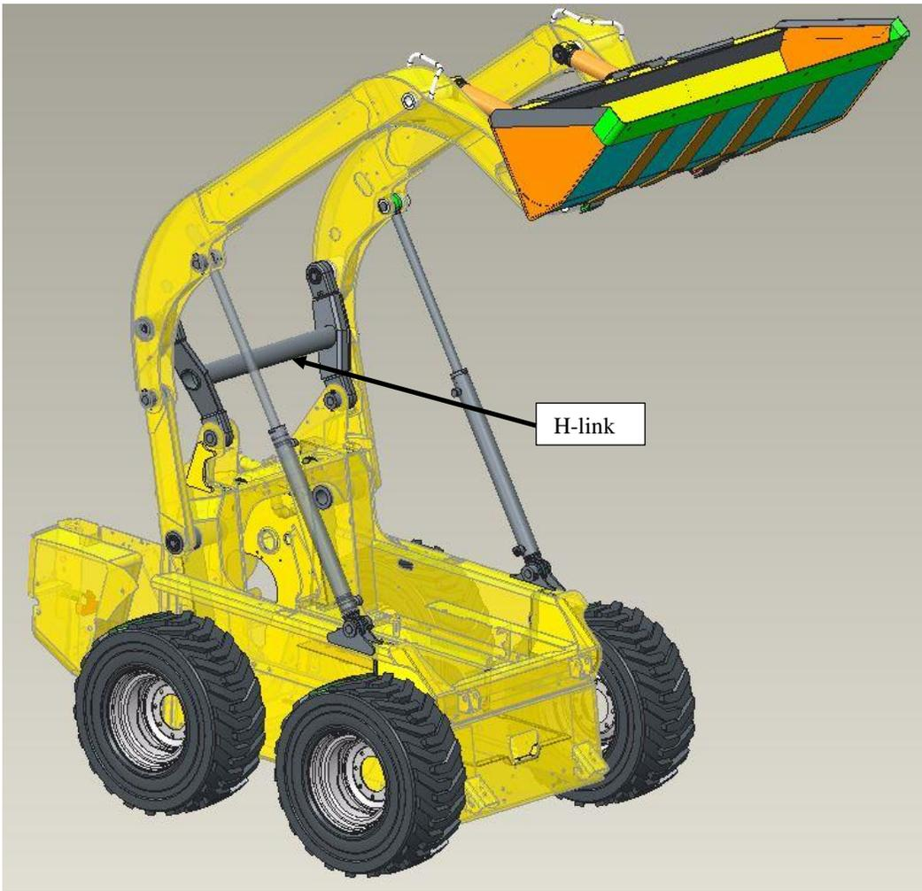
**Figure 1. CAD model of vertical lift loader assembly on chassis.**
