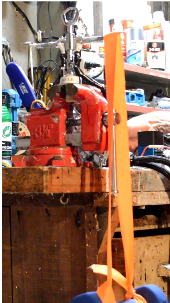
Figure 11: Corkscrew dead weight calibration test.
