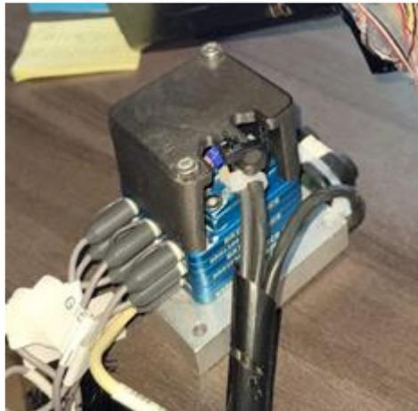
**Figure 4: DTS Slice Micro DAQ**
